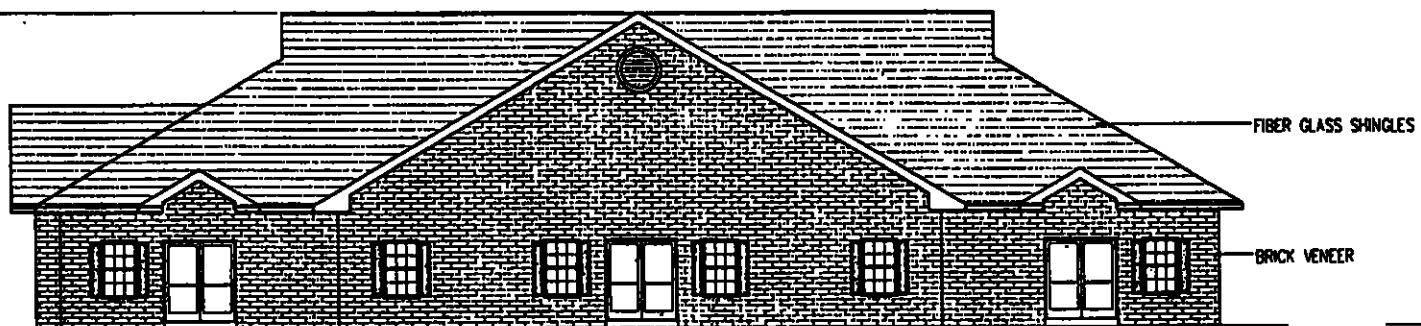
FRONT ELEVATION (EAST ELEVATION) SCALE: 1/8" = 1'-0"
