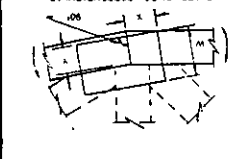
PB2(N) 90° PLATE LENGTH PERPENDICULAR TO CHORD
