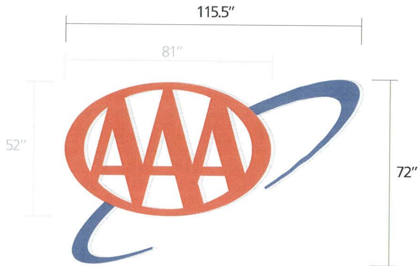
FRONT ELEVATION - Sign Type (A.1)(QTY:1) Channel Letter / Logo - Remote Mount Scale: 3/16" = 1' (57.75 SQFT)
