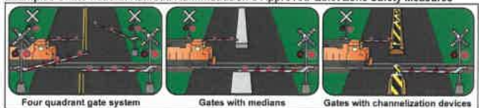
Examples of the Federal Railroad Administration's Approved Quiet Zone Safety Measures
