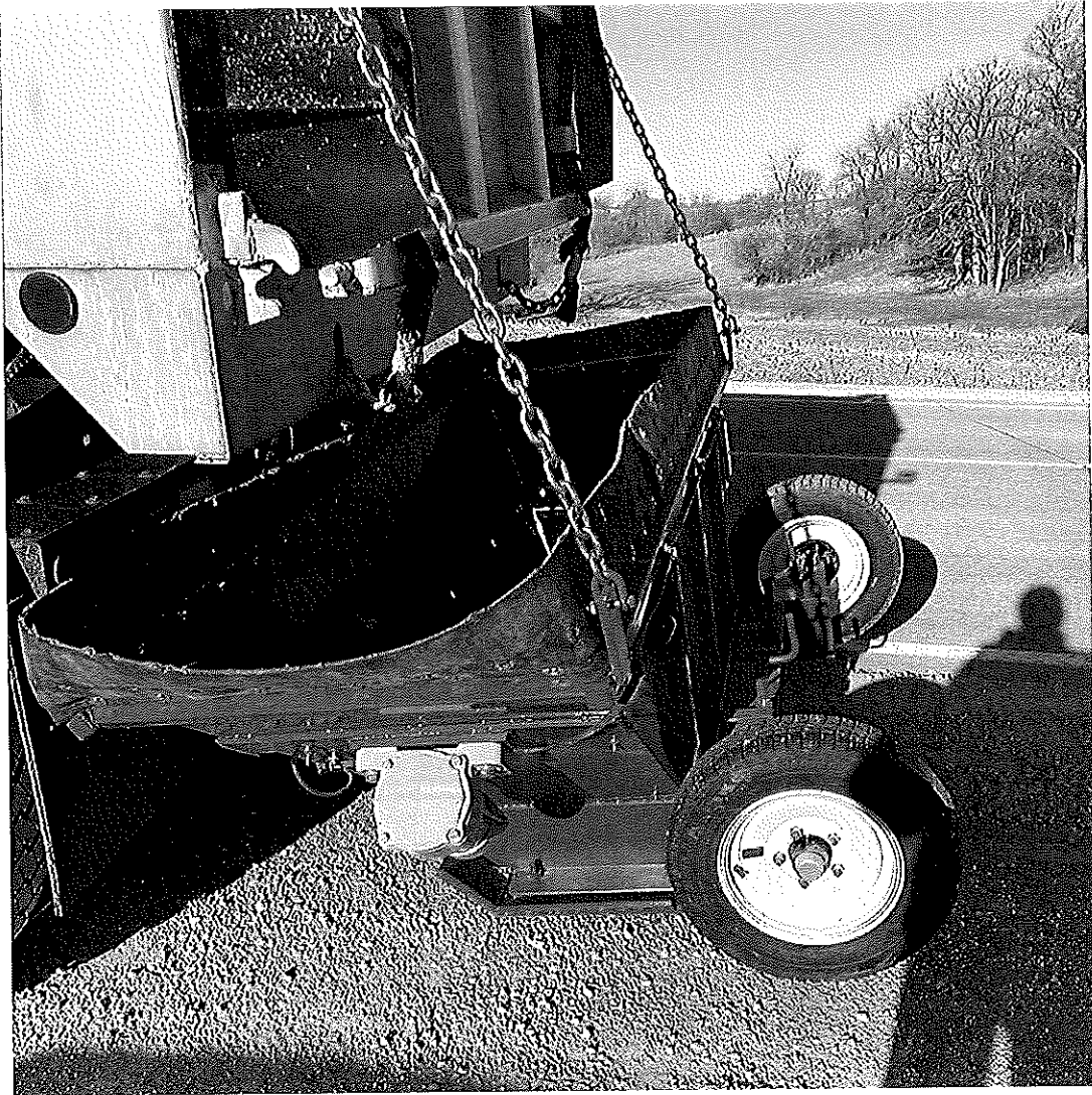
Photo credit: Jones County, IA. Pictured is the Hopper innovation created in Jones County, IA to improve shoulder maintenance.
